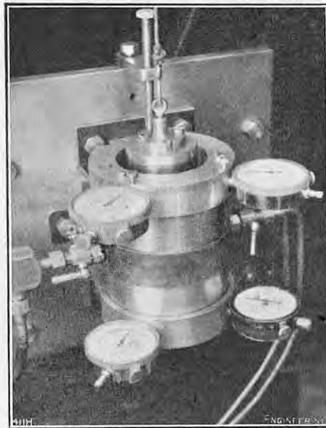
FIG. 10. ARRANGEMENT OF DIAL GAUGES.
