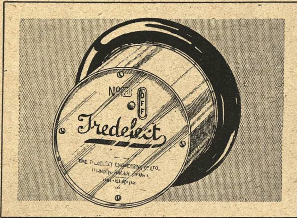
The charging indicator, which is fitted to the dash.
