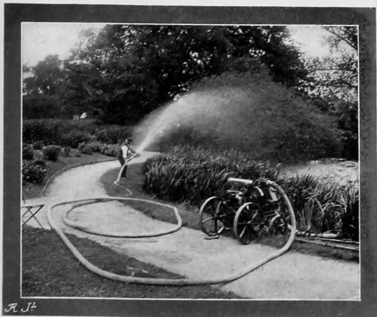
FIG. 1.—The Merryweather "general purposes" pump at work in the Grounds of the Botanical Gardens.
