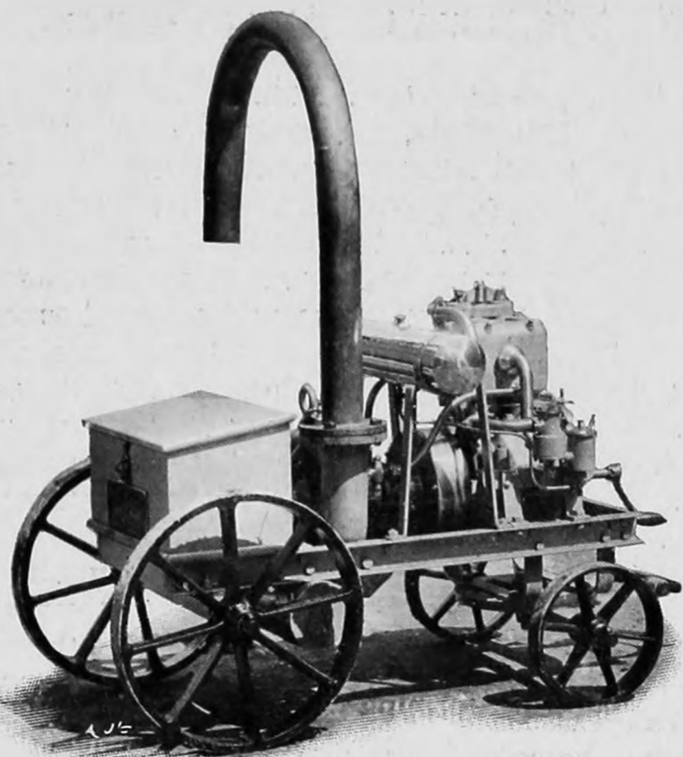
FIG. 3.—A compact Petrol Motor-Driven Centrifugal Pumping Plant, specially constructed by Messrs. Merryweather and Sons for irrigation purposes.
