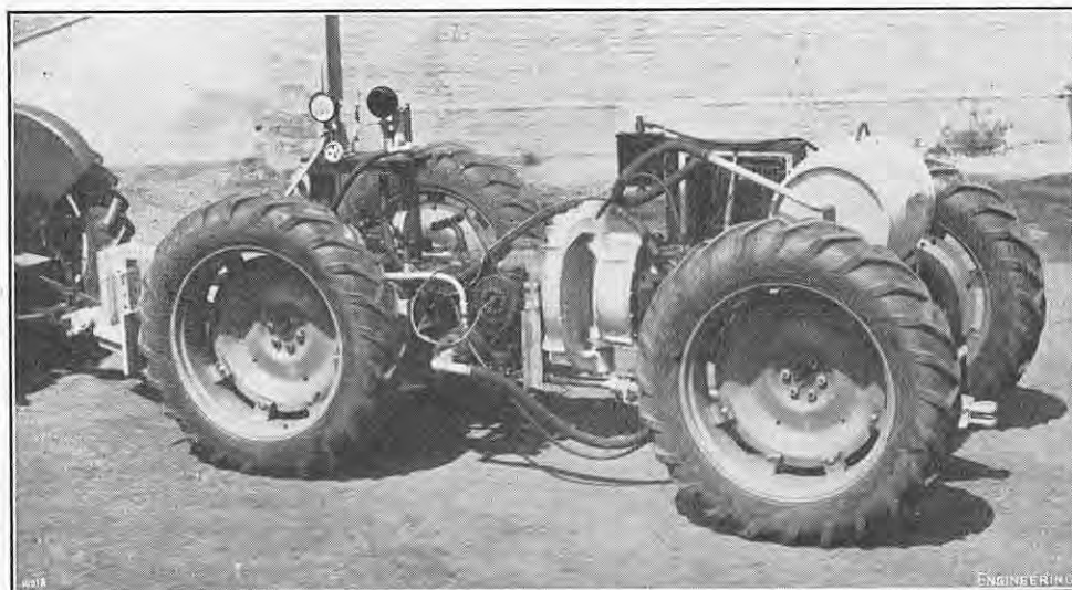
FIG. 5. HYDRAULIC CAR FOR LOADING TRACTOR DRAWBARS.
