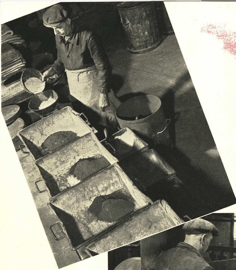
WEIGHING UP. The compounds for hundreds of mixings are accurately weighed before being incorporated into the rubber.
