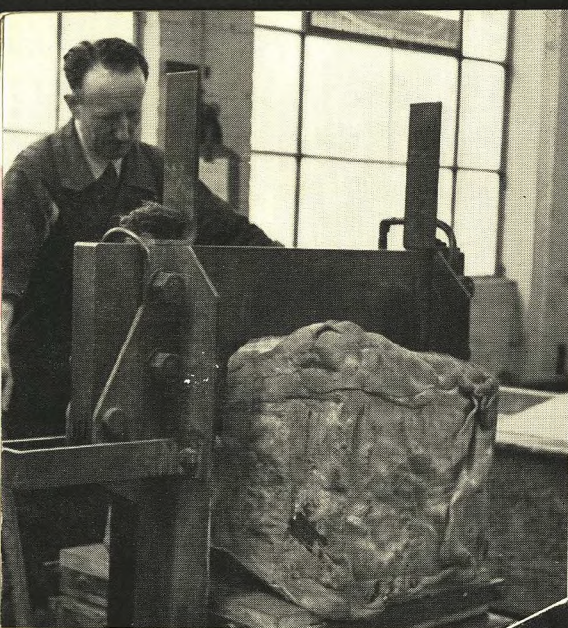
THE BALE CUTTER AT WORK. When J. G. Ingram first began one hundred years ago, he had only small supplies of wild Para to work on. Now, most of the rubber comes from Malaya and the photograph illustrates a 225-lb. bale of Malayan Smoked Sheet being forced against the cutting knife by a very powerful hydraulic-operated platform.
