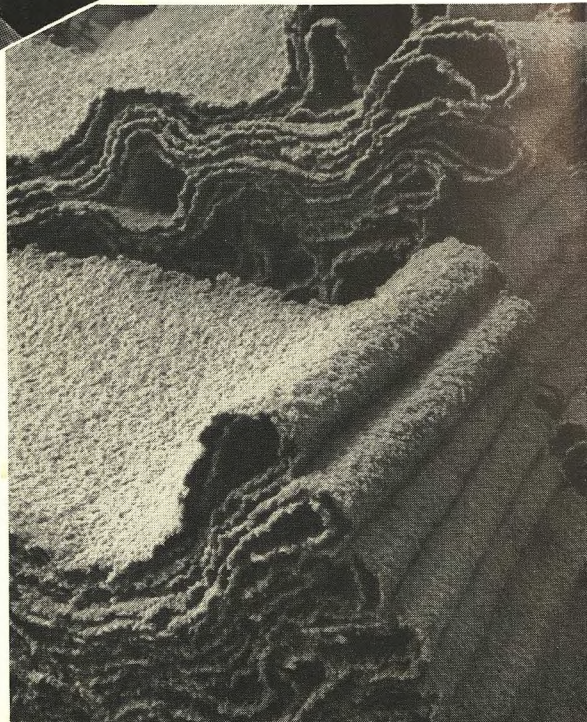
WASHED RUBBER. The first stage of manufacture has been completed. The washed rubber is in sheet form, ready for the drying machine.
