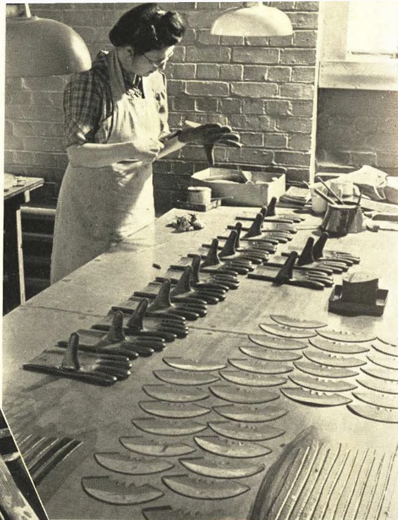
TESTED UP TO 10,000 VOLTS. Hand-made Electrical Gloves.
