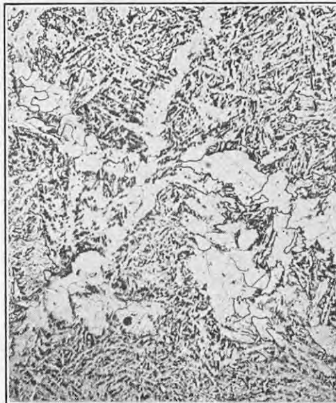
FIG. 2. HOT-DRAWN CR-MO STEEL. \times 150 .
