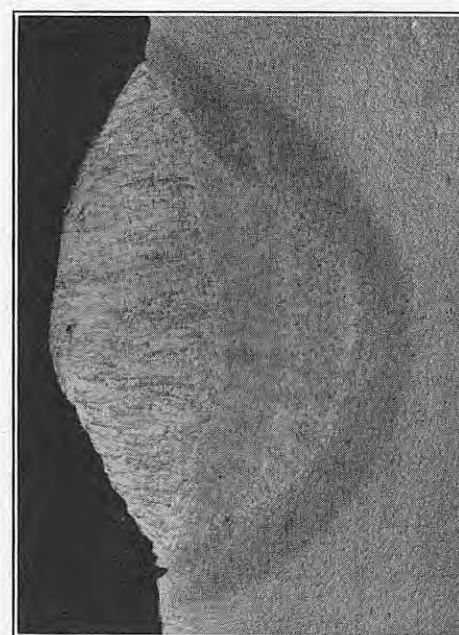
FIG. 11. COLD-DRAWN MO-V STEEL AFTER 350 HOURS AT 625 DEG. C. × 5.
