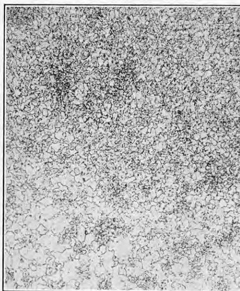
FIG. 10. HEAT-AFFECTED ZONE OF WELD. MO-V STEEL AFTER 350 HOURS AT 625 DEG. C. × 150.
