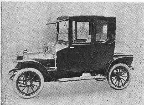
A neat little coupe body fitted to a Zedel chassis. As will be noticed it is fitted with a boat-bow dash, and is altogether as snug as a car can well be.
