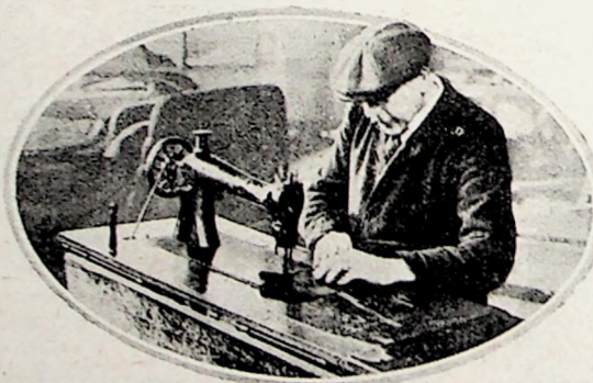
An ordinary sewing machine is suitable for working upon even such thick materials as leather cloths, provided that strong needles and threads are used.
