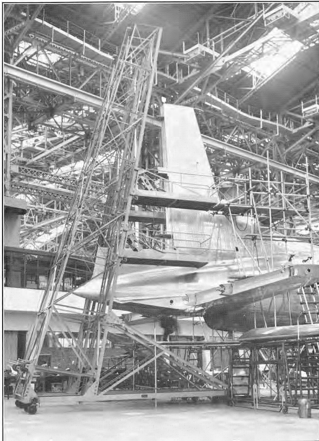
FIG. 20. SERVICING TOWER FOR FIN AND RUDDER.
