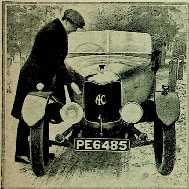
There are no bonnet fasteners of the usual kind. "Lift and pull" is the formula to be followed for obtaining access to the engine. Hartford shock absorbers are fitted at the front, as can be seen in this photo.
