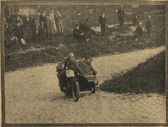
On Thwaites Brow in the Ilkley M.C. and L.C. Club's trial. The left-hand turn requires careful negotiation with a motorcycle combination as the sidecar has a tendency to rise. But—
