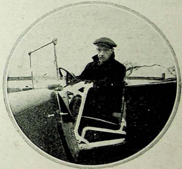
— access is gained to the rear seats by a neatly folding front near-side seat. The body is deep, affords good protection, and has one door only.
