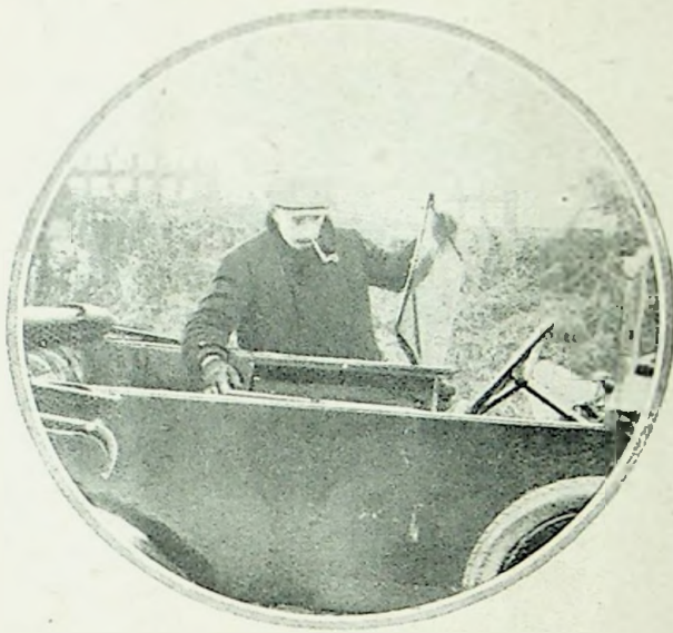
These two photographs reveal a degree of comfort typical of the whole car. As the sidescreens are carried in the walls of the single shell body, their erection does not disturb passengers, whilst
