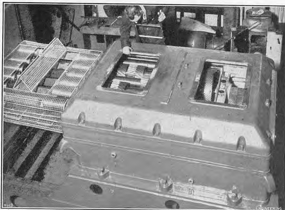
FIG. 2. GEARBOX, SHOWING OIL GALLERY.
