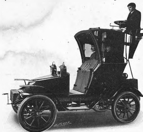
A Vauxhall 9 h.p. three-cylinder standard chassis carrying a hansom cab body. As can be seen the steering and control gear are taken up to the driver, who sits in the usual hansom cabdriver's position. A number of the cabs are being built to the order of the Metropolitan Motor Cab and Carriage Co. by the Vauxhall and West Hydraulic Eng. Co., Ltd., of 45 Leadenhall Street, and of Luton
