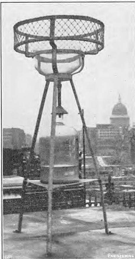
FIG. 7. DEPOSIT GAUGE FOR MEASURING ATMOSPHERIC POLLUTION.
