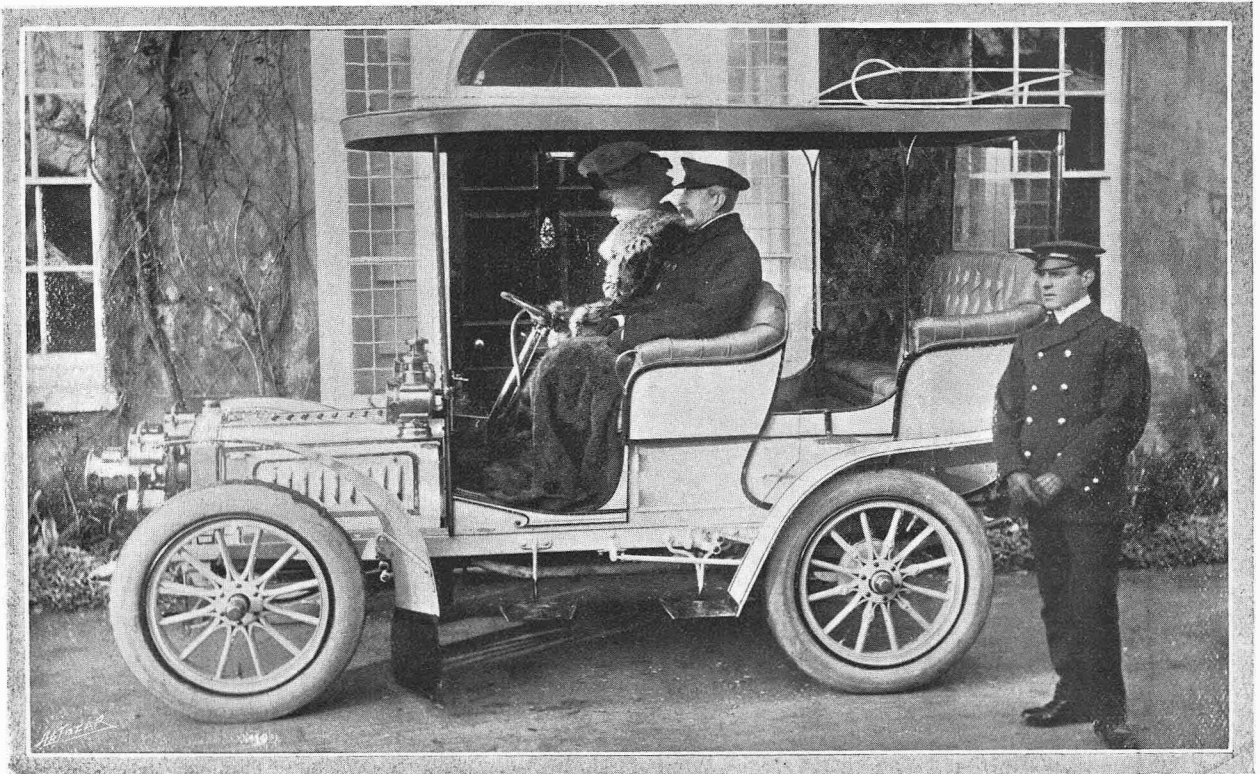
A HANDSOME CAR. Enthusiastic automobilists are Co. F. C. Ord and Mrs. Ord, of Bristol. Although comparatively new converts to automobilism, they have already had a 14 h.p. Daimler and a 20 h.p. Talbot, which latter vehicle we illustrate. The main intent of the body design is to combine detachable top and side entrance to the back seats without lengthened wheelbase. This is done very neatly, and it will be observed that a step is provided above the rear mudguard so that Colonel Ord's man can get into the car without opening the side entrance. 120 mm. tyres are fitted to all four wheels, as the owner of the car thoroughly realizes the value of the large tyres. In our illustration, Mrs. Ord is shown at the wheel with Colonel Ord by her side.
