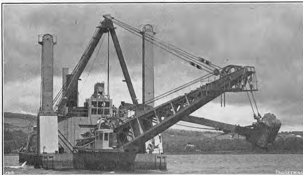
FIG. 7. DIPPER DREDGE "KALA NAG."
