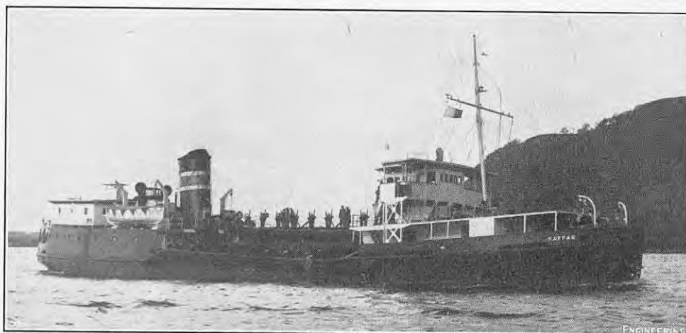
FIG. 9. TRAILING-SUCTION HOPPER DREDGE "HAFFAR."
