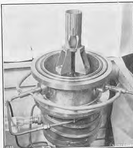
FIG. 2. GRAPHITE HEATING ELEMENT FOR HIGH-VACUUM FURNACE; GENERAL ELECTRIC COMPANY, LIMITED.
