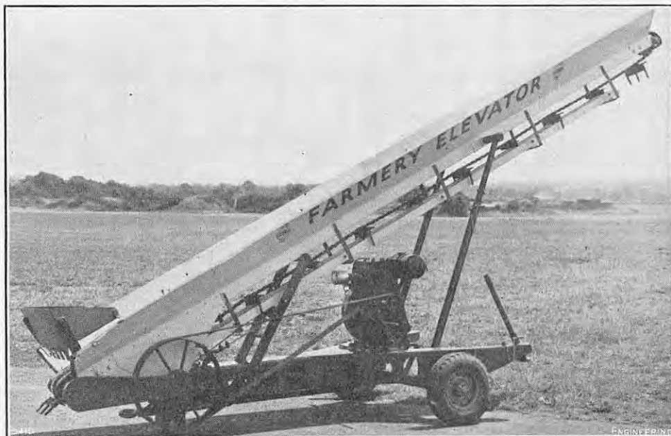
FIG. 4. BALE ELEVATOR; ALPEMA AGRICULTURAL DEVELOPMENT COMPANY, LIMITED.
