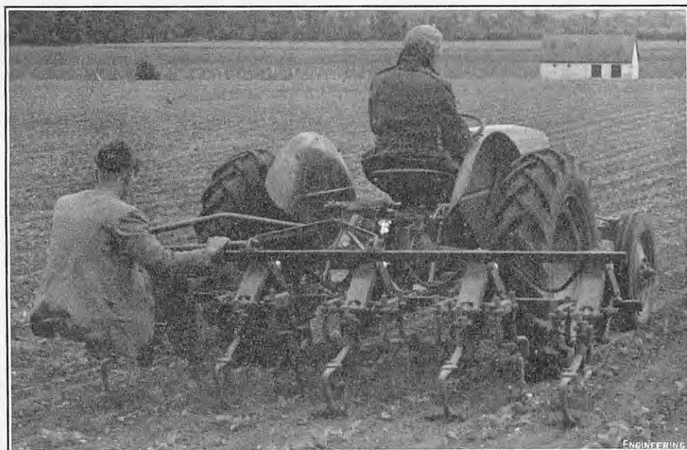
FIG. 5. INDEPENDENT GANG STEERAGE HOE; HARRY FERGUSON, LIMITED.
