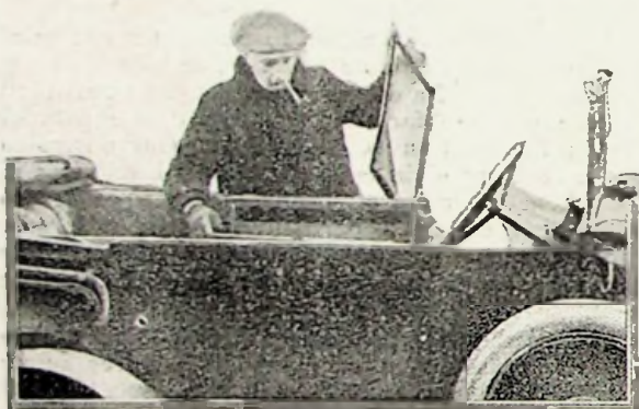
A popular way of storing the side screens. Capacious pockets are provided in the sides of the car. Passengers need not be disturbed to withdraw the screens.
