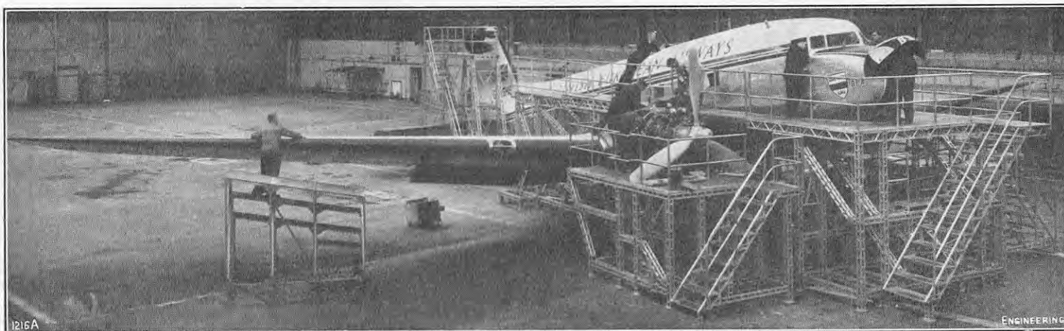
FIG. 1. "PIONEER" AIRCRAFT BEING SERVICED.
