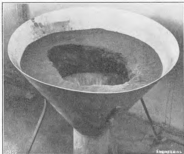
FIG. 2. ARRESTED FLOW OF PEAT IN A FUNNEL.
