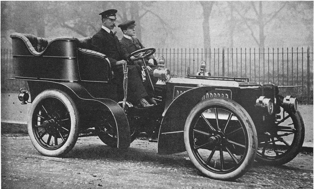
A HANDSOME CAR. The illustration above depicts a 24-hp. De Dietrich supplied to the order of Mr. J. Hamilton Houldsworth, of Coltness Castlebank, Lanark. The body, which was constructed by the Burlington Carriage Co., 315 and 317, Oxford Street, W., has been designed with a special view to the requirements of the owner. The tonneau provides accommodation for five persons, two of the seats being removable when the car is set upon the road in touring trim. The vehicle is upholstered in fine English leather, harmonising with Mr. Houldsworth's family colours in which the body is finished. These are a taking Brunswick green, with lighter green relief. The automobilist at the wheel is Mr. A. S. Mays-Smith, the general manager of the Burlington Carriage Co., who made a careful test of this beautiful car before it was delivered to Mr. Houldsworth. Mr. Mays-Smith was the first man to recognise the merits of and place a four-cylinder De Dietrich on exhibit in any London showroom. In the interest of those of the Burlington Carriage Co.'s clientele who are supplanting their horse-drawn vehicles by motor cars, Mr. Mays-Smith has been at some pains to have at the Dietrich works a staff of mechanics carefully drilled in the mechanism and economy of these cars.
