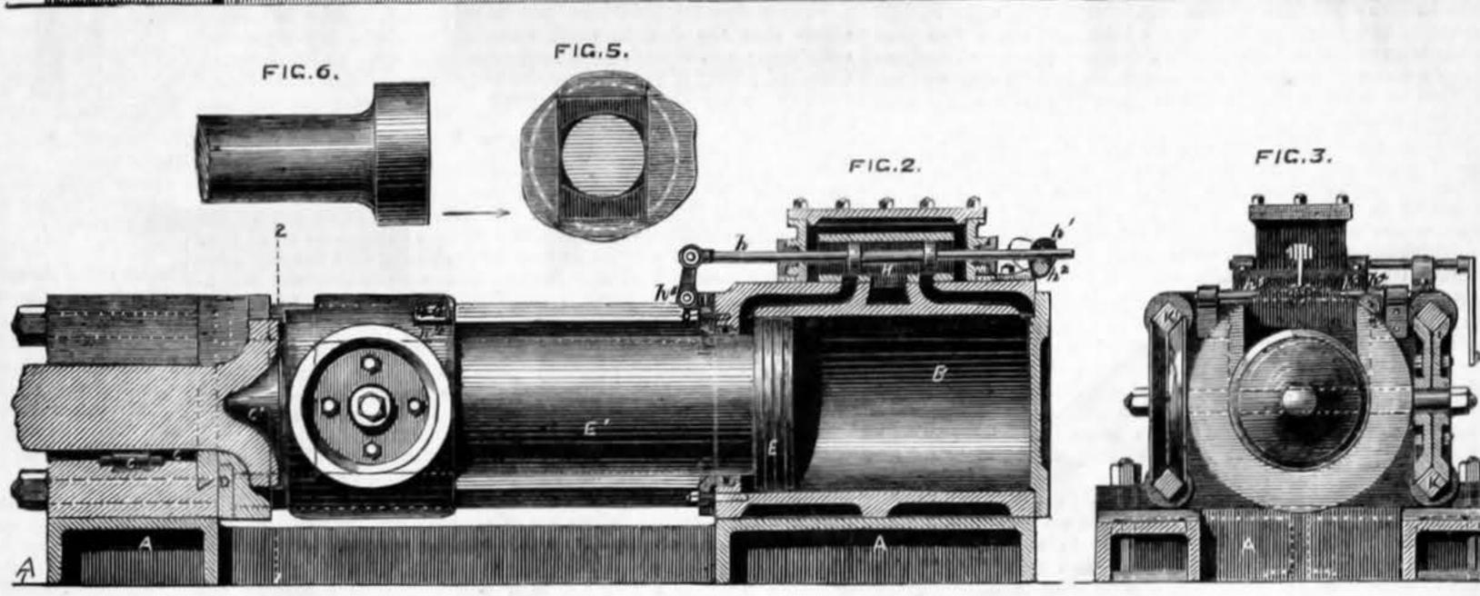
cause the valve to advance and cut off the supply of steam to the cylinder, while at the same time it will stop the escape of the exhaust steam, and thus provide an elastic cushion for the piston to strike against.
