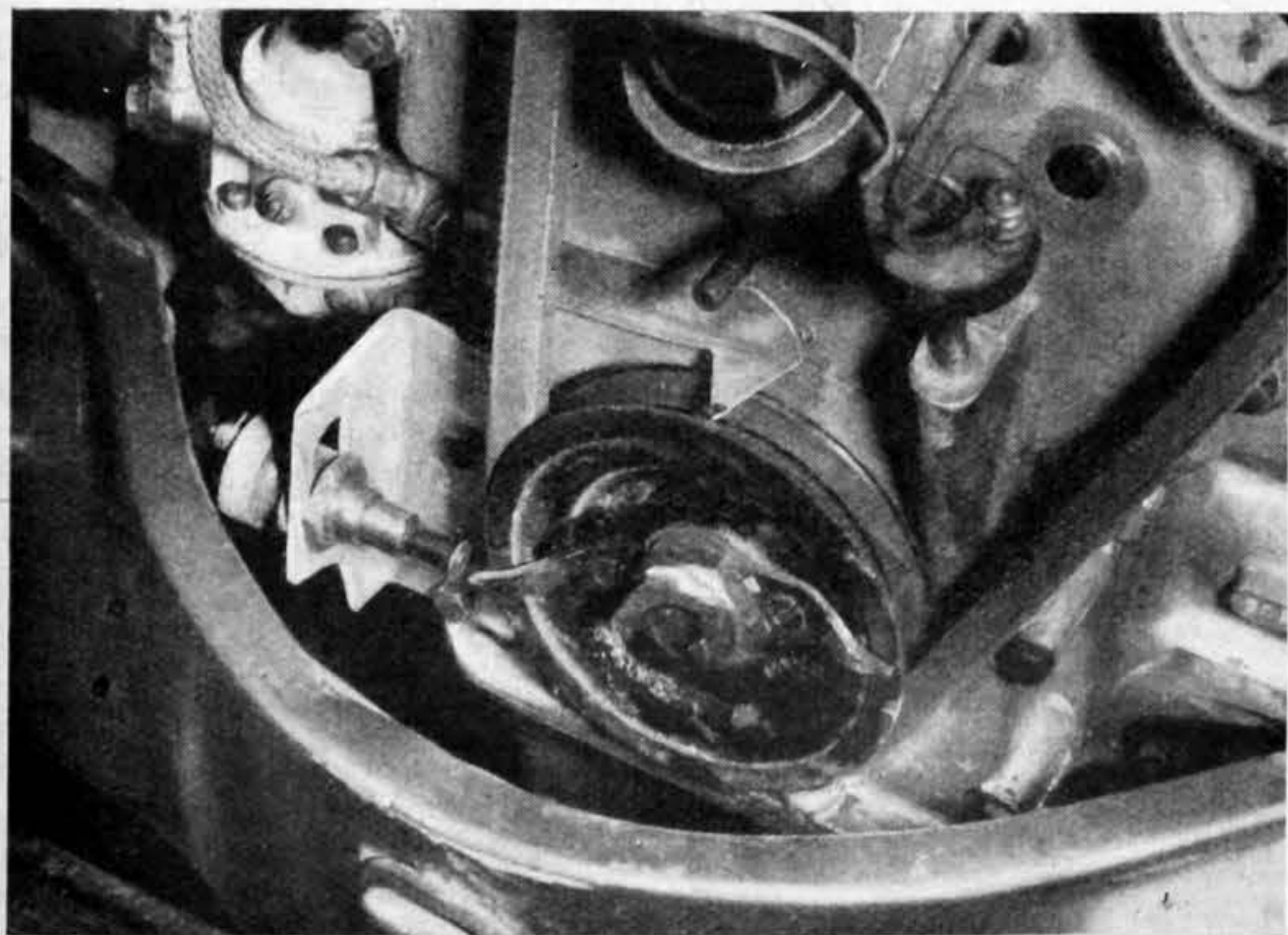
FIG. 2—ELECTROMAGNETIC PICK-UP INSTALLATION
