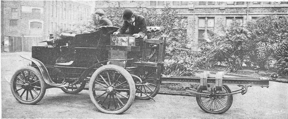
The car with the tractive resistance recording instrument attached. It will be noticed that a voiturette type wheel is in the frame. Note the number of weights as compared with the heavier load on the wheel below.
