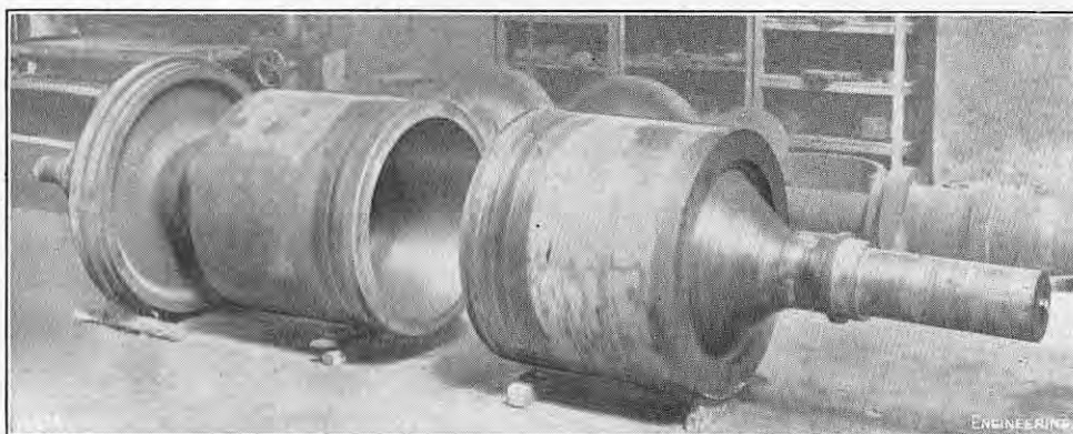
FIG. 18. STEAM-TURBINE ROTOR COMPONENTS BEFORE WELDING.
