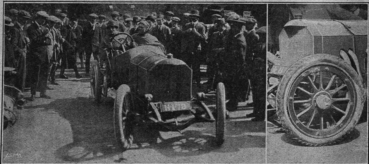
Two views of Mr. A. W. Tate's Mercedes which skidded and struck an iron fence near the start. Both views of the car were taken after the accident, and it will be noticed that a front wheel hub cap which was crumpled up in scraping the fence has been replaced by the top of a loaf of bread to keep out the dust and retain the lubricant.
