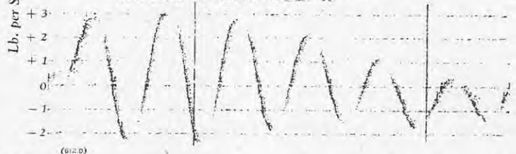
Fig. 8. CORRESPONDING EXHAUST-PRESSURE DIAGRAM PRODUCED BY FARNBORO'
