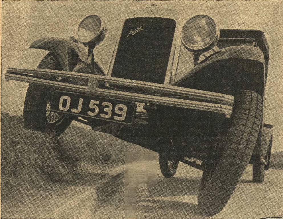
You would not do this from choice, but here is an untouched photograph of an Austin car purposely driven into this position to show the sort of stress which the new cross-braced frame is built to stand.
