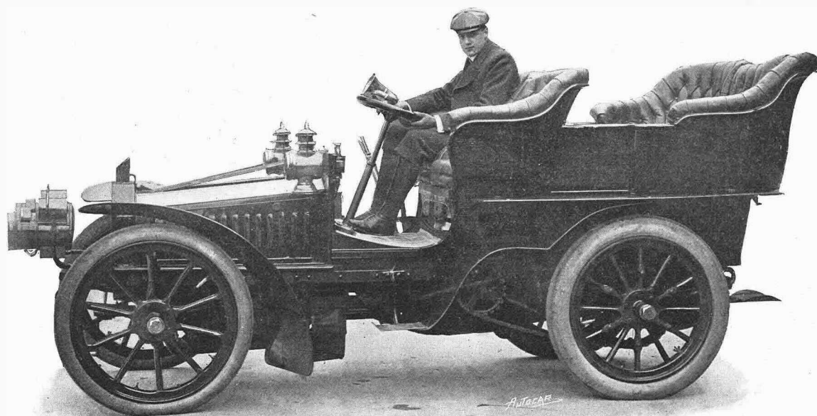
This vehicle is a standard pattern 20 h.p. Milnes, built for Mr. L. Fleischmann. It is fitted with a Rothschild body, and is interesting as showing the tendency to make the two rear seats of the tonneau even more luxurious and comfortable than the double scolloped front seat.
