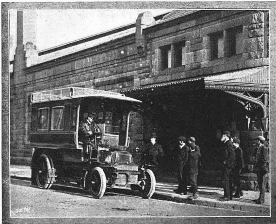
THE G.W.R. MOTOR SERVICE. One of the Great Western Railway Co.'s 16 h.p. Milnes-Daimler omnibuses outside Penzance Station. These vehicles accommodate twenty-two passengers and carry a certain quantity of luggage on the roof. The front wheels are shod with Goodyear solid tyres, the back wheels having twin Sirdar Buffer tyres. Side by side with this is given a reproduction of the official time table, which is one of the first dealing with motor vehicles to be issued by any main line railway. We are indebted to Mr. S. W. Taylor, of Penzance, for the photograph from which our illustration is reproduced.
