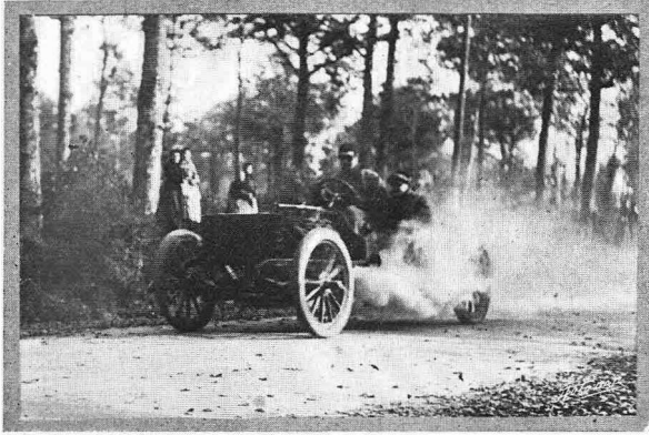
A competing car at full speed. The smoke issuing from the side is the result of an overdose of lubricating oil.
