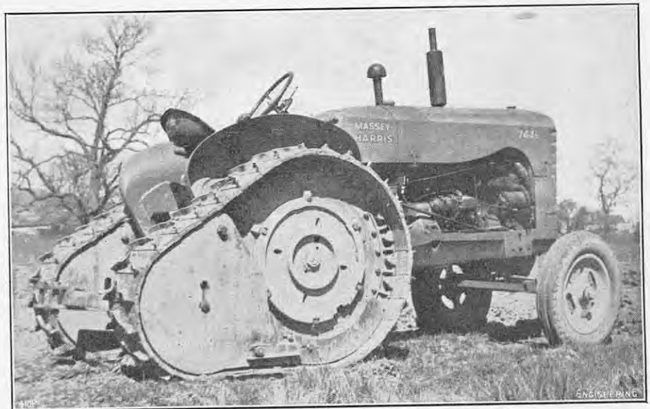
FIG. 13. HALF-TRACK CONVERSION; MESSRS. JAMES A. CUTHBERTSON, LIMITED.
