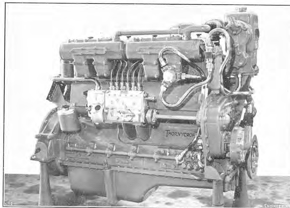
FIG. 36. 125-B.H.P. INDUSTRIAL DIESEL ENGINE; JOHN I. THORNYCROFT AND COMPANY, LIMITED.
