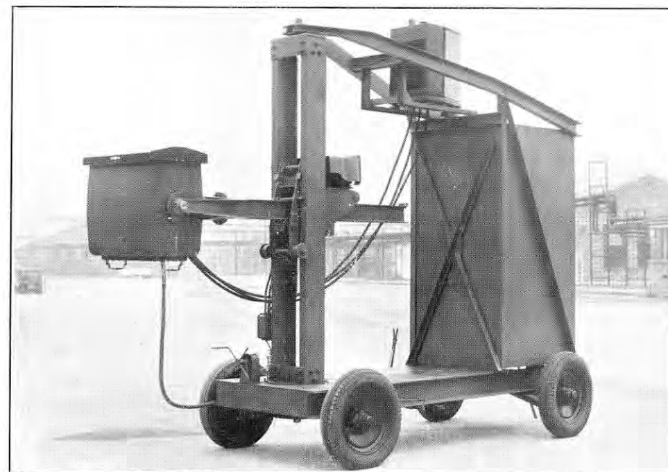
FIG. 48. 250-KV INDUSTRIAL X-RAY EQUIPMENT ; NEWTON VICTOR, LIMITED.
