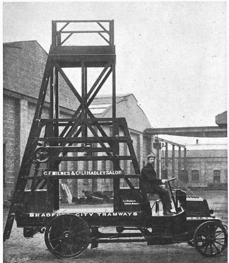
The Milnes-Daimler motor telescopic tower supplied to the Bradford City Tramways for the repairing of the overhead trolley wires. On this vehicle all tools and other requisites are carried, and breakdowns can be attended to very much more speedily than with the old horse-drawn apparatus.
