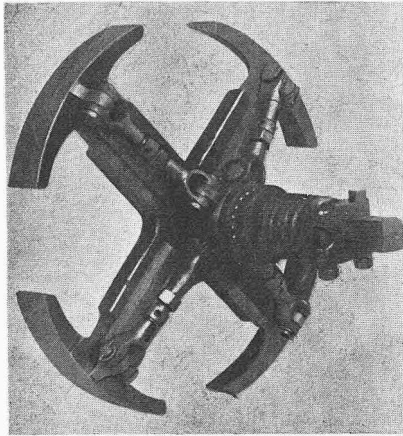
The new Clément expanding clutch.
