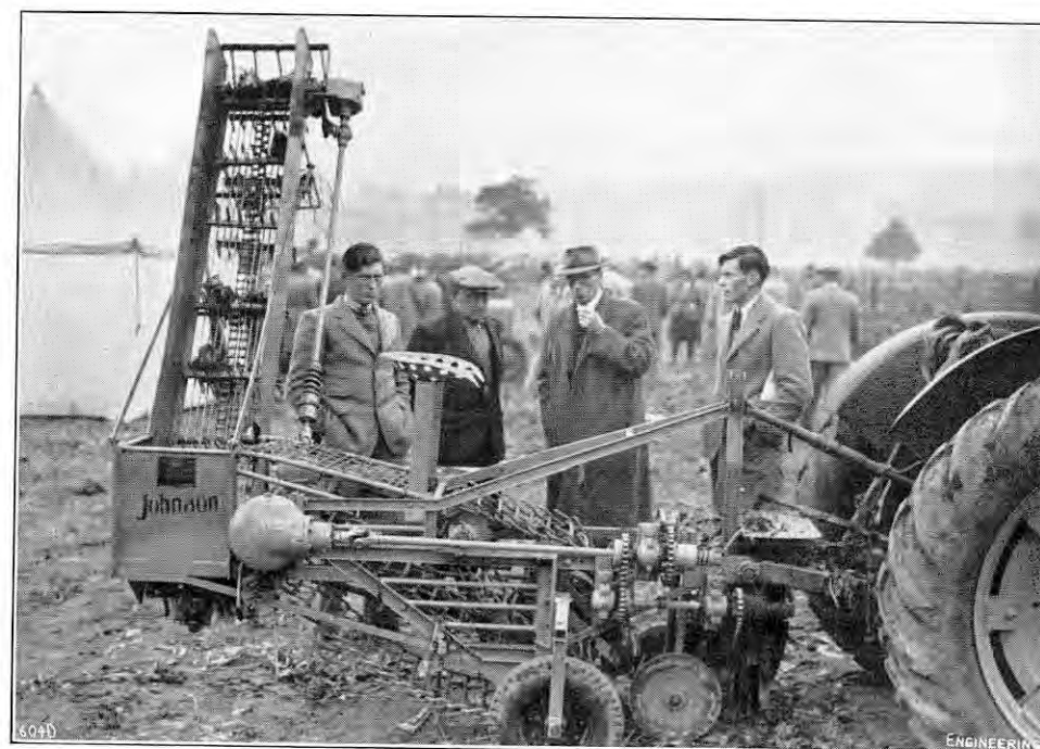
FIG. 4. TRACTOR-MOUNTED SUGAR-BEET HARVESTER; JOHNSON'S (ENGINEERING), LIMITED.
