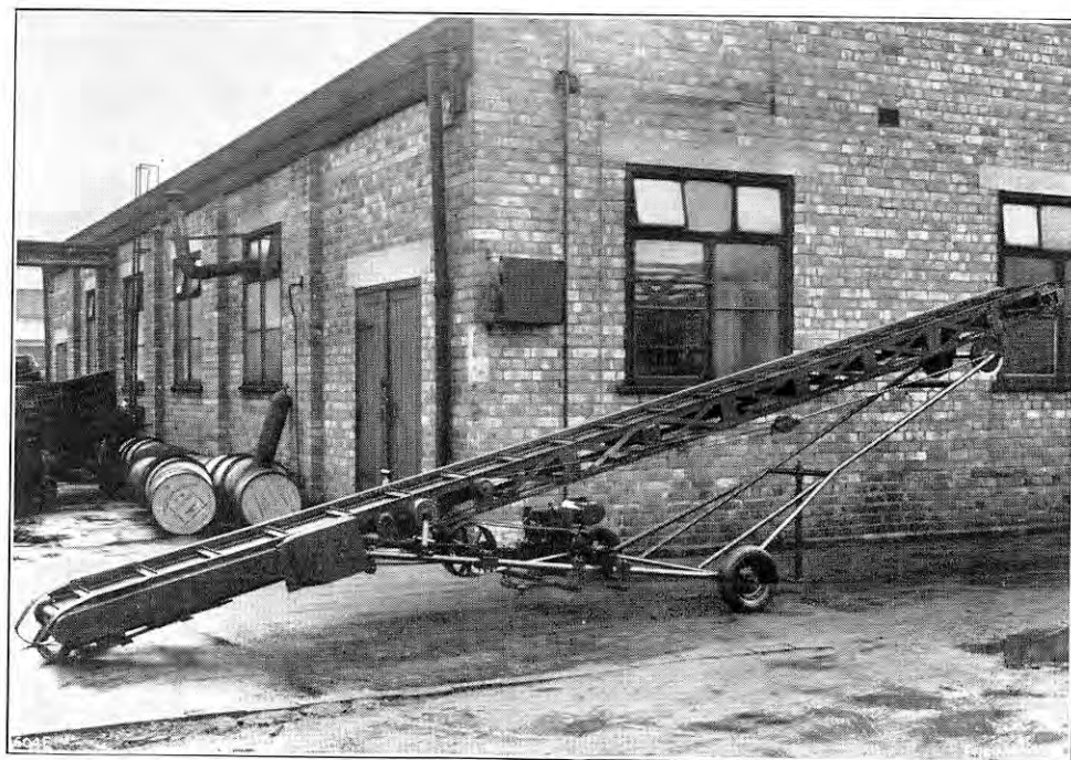
FIG. 5. VARIABLE-HEIGHT ELEVATOR; WOLSELEY SHEEP SHEARING MACHINE COMPANY, LIMITED.
