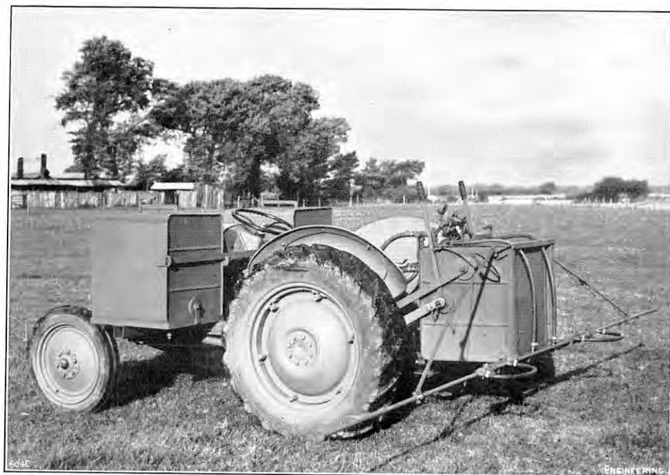
FIG. 3. TRACTOR-MOUNTED CROP SPRAYER; E. ALLMAN AND COMPANY, LIMITED.
