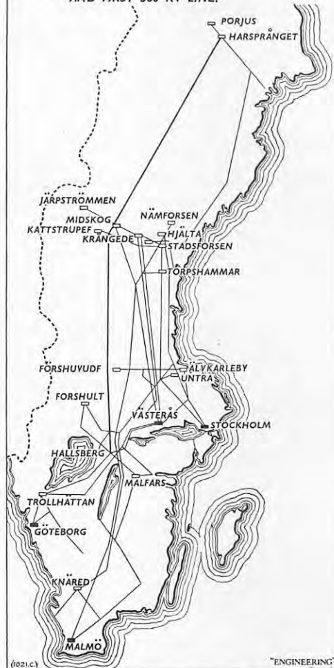
Fig. 2. 220 AND 130-KV SYSTEMS AND FIRST 380-KV LINE.
