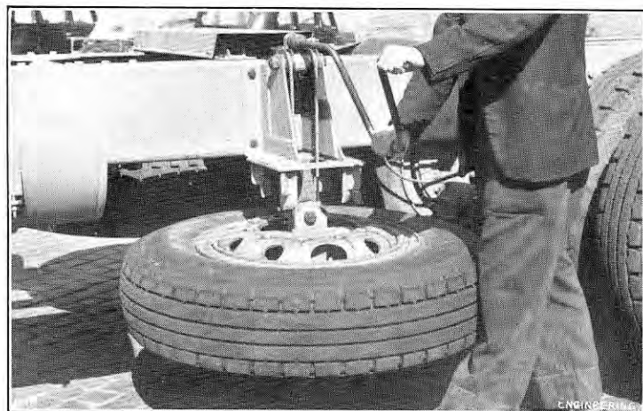
FIG. 28. SPARE-WHEEL HOIST ON "TRUSTY" CHASSIS.
