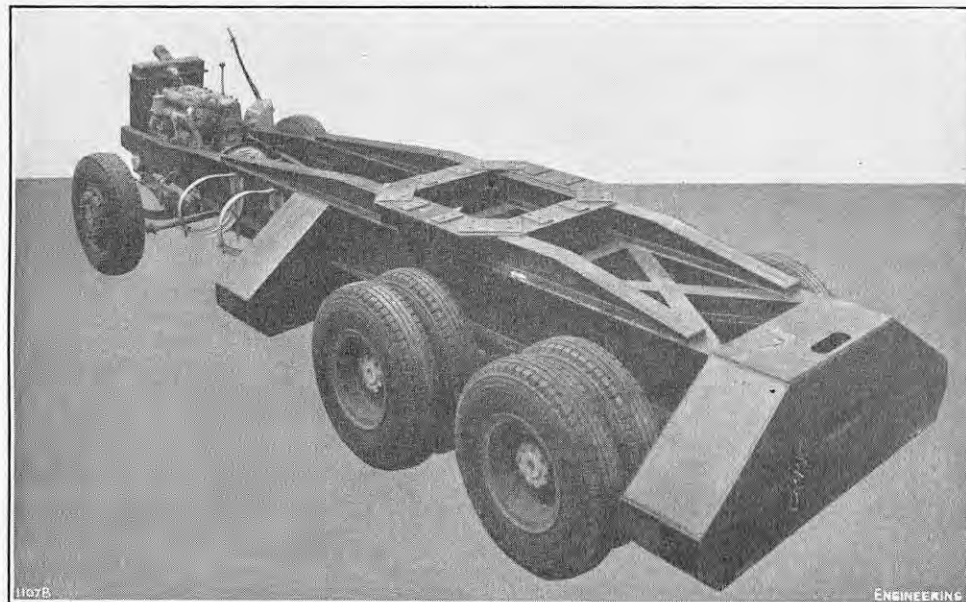
FIG. 1. CRANE CHASSIS, WITH LEYLAND "HIPPO" COMPONENTS.
