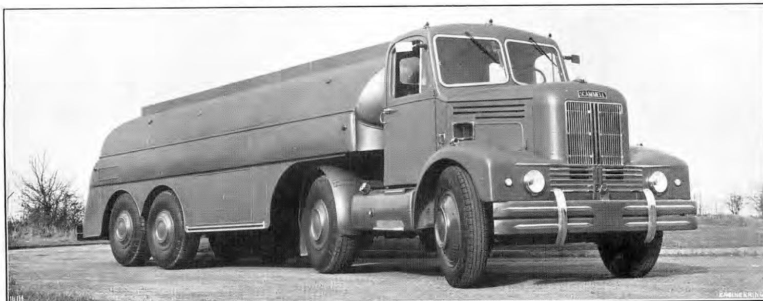
FIG. 26. TRACTOR AND SEMI-TRAILER FOR BULK TRANSPORT OF LIQUIDS; SCAMMELL LORRIES, LTD.
