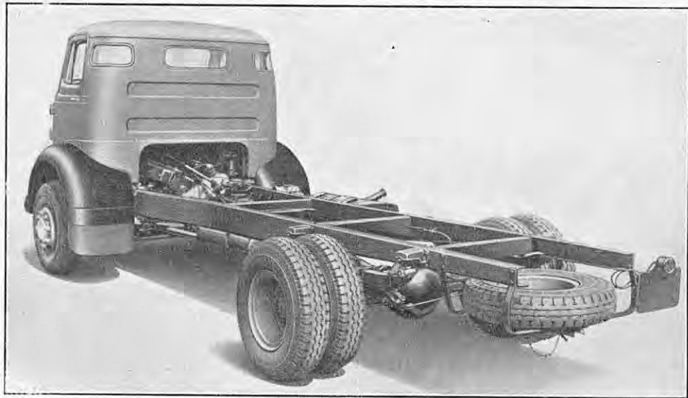
FIG. 19. LOAD CARRIER WITH UNDERFLOOR ENGINE; KARRIER MOTORS, LTD.
