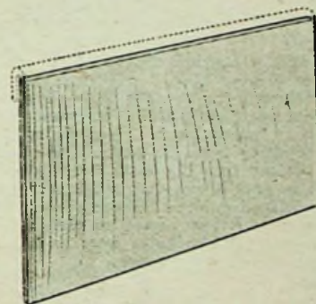
When cutting very thin sheet metal it may be folded over as above and the part shown by the dotted lines filed off. This method prevents buckling.
