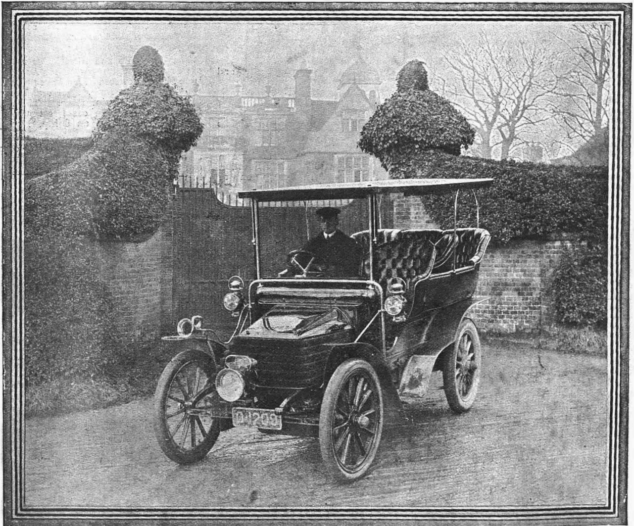
Lord Hindlip's handsome 24 h.p. Wolseley car. It is fitted with a long double tonneau body with "rullip" seats moulded in aluminium, painted dark red, lined light red and white lines, and upholstered to match. A departure from the usual "Wolseley" practice is the fitting of a curved dash on which is mounted a plated rail, which greatly adds to the car's appearance; this rail is extended to serve as a support for the front portion of the canopy, where a glass weather screen is also fitted.
