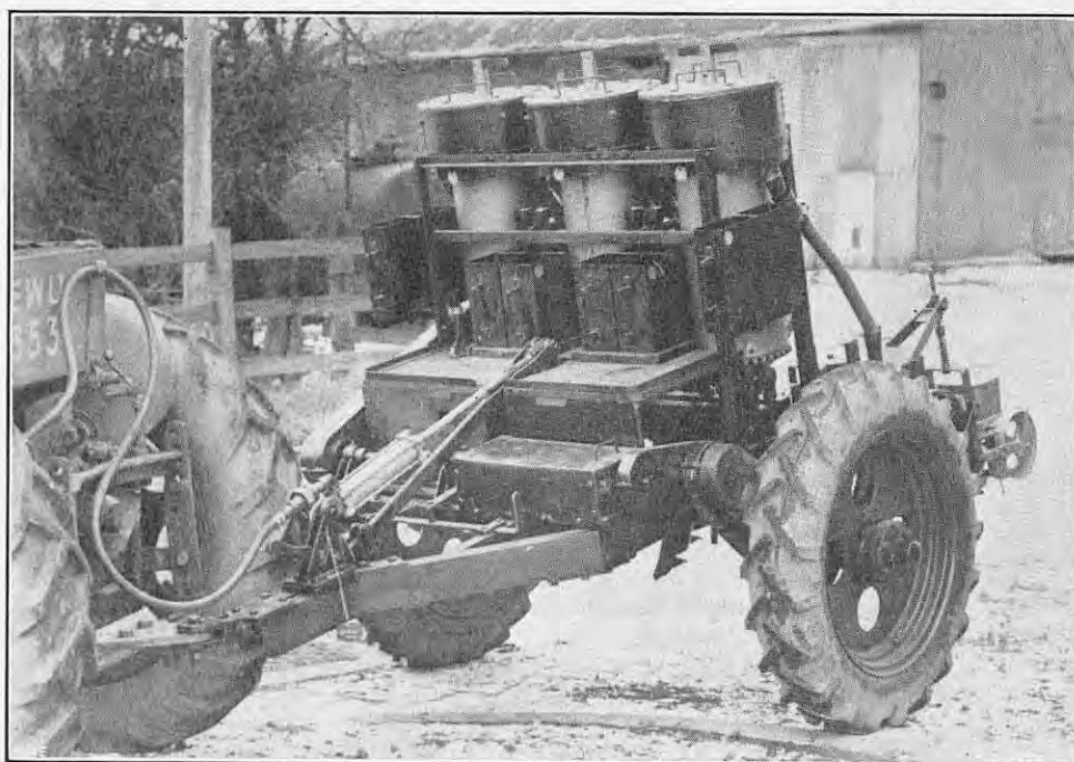
FIG. 5. FERTILISER-PLACING MACHINE WITH HYDRAULICALLY-ACTUATED CRANKED AXLE.
