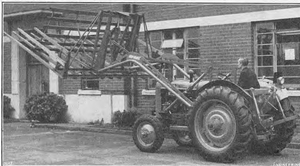
FIG. 2. NUFFIELD TRACTOR FITTED WITH STRIPPING FORK.
