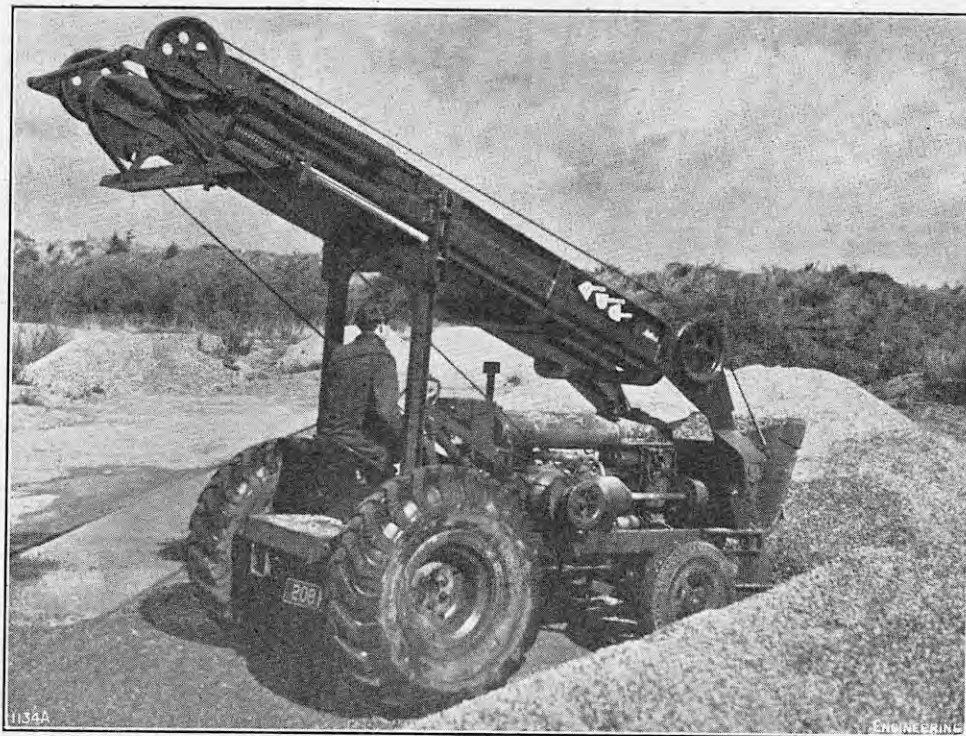
FIG. 1. OVERHEAD LOADER; MACKAY INDUSTRIAL EQUIPMENT, LTD.
