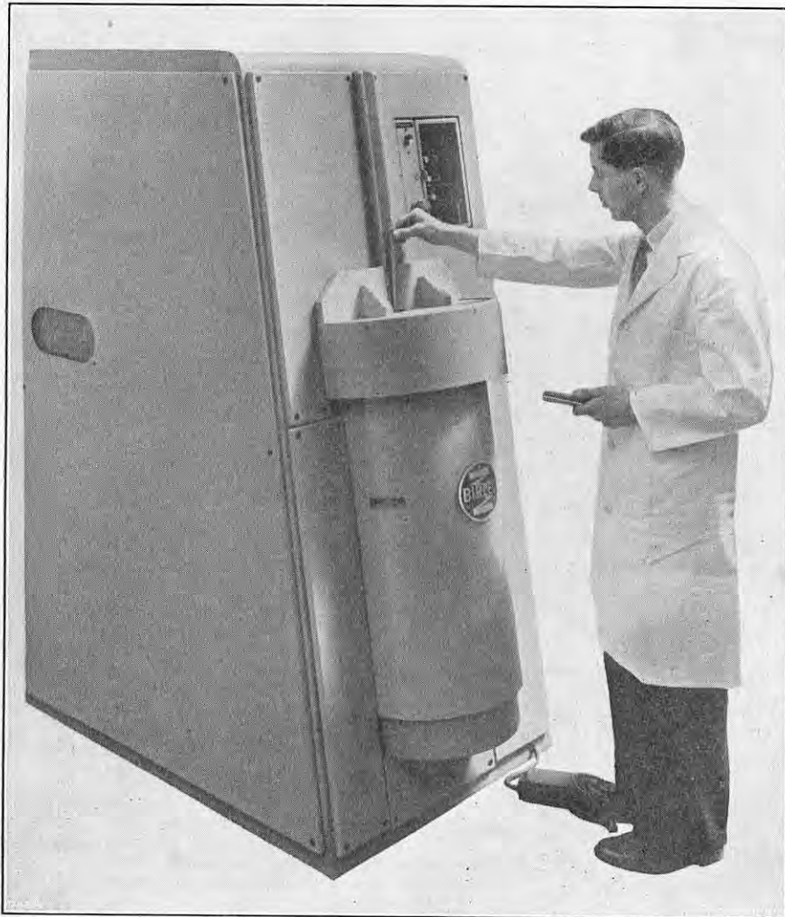
FIG. 1. LOADING SHAFT INTO HEATER.
