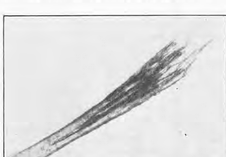
FIG. 5. WOOL FIBRE, FIBRILLISED IN LABORATORY TEST (REF. 4.) \times 125 .
