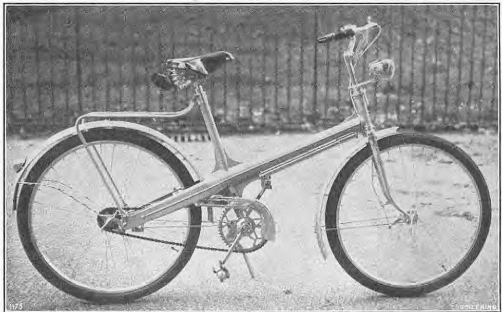
BICYCLE WITH ONE-PIECE ALUMINIUM-ALLOY FRAME.
