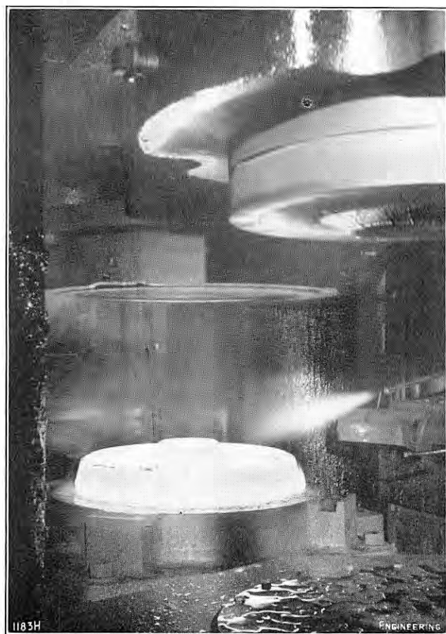
FIG. 12. FORGING PRODUCED IN 8,500-TON PRESS.
