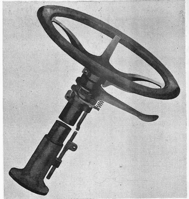
Fig. 3.—N.E.C. tilting steering wheel showing all round throttle lever.
