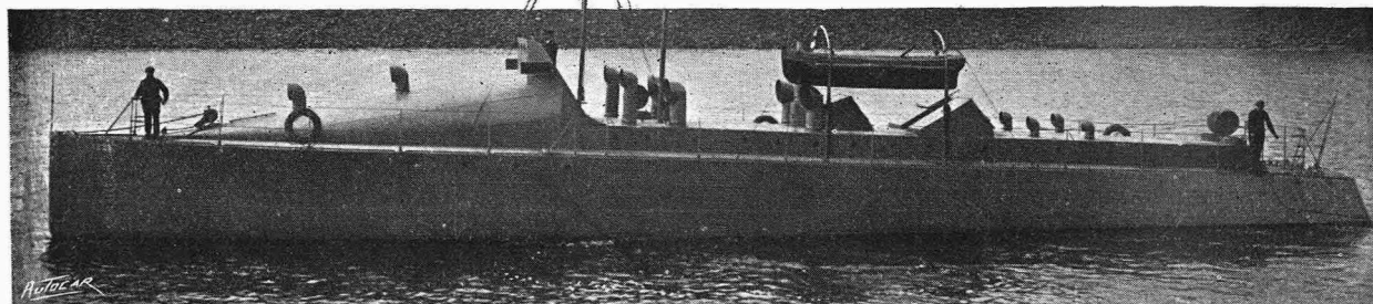
A smart high speed sea-going torpedo boat or gunboat built by Messrs. Yarrow and Co., Ltd. She is 100ft. long and 13ft. 6in. beam, and is equipped with a 600 h.p. set of six-cylinder Napier engines, driving four propellers. The new boat is 40ft. longer and 4ft. 6in. greater in beam than the famous Yarrow-Napier of 1906, while her engines are double the power of that boat. At 21 knots her radius of action is 300 knots, at half speed 600 knots. The saving in weight and space, as compared with a steam engine of equal power, amounts to some 50 per cent.
