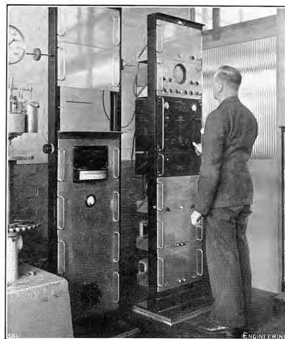
FIG. 14. DETERMINATION OF YOUNG'S MODULUS BY RESONANCE.
