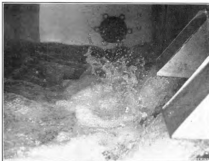
FIG. 26. TURBULENCE IN DUMMY BOILER DRUM.
