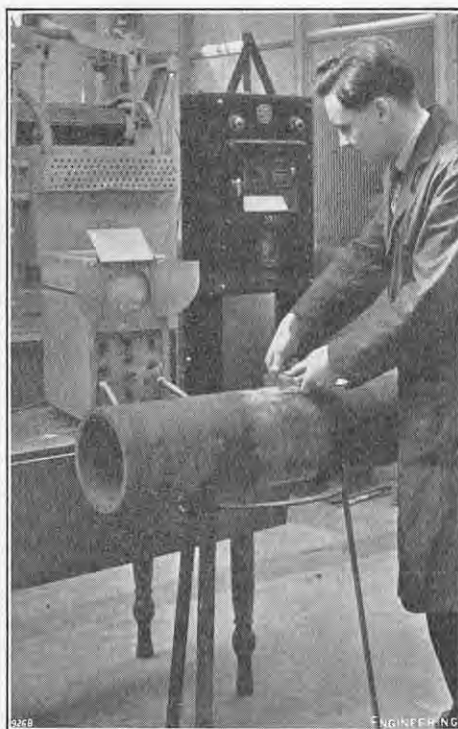
FIG. 2. ULTRASONIC TEST OF BUTT-WELDED PIPE JOINT.
