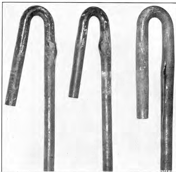
FIG. 13. SUPERHEATER TUBES TESTED TO FAILURE.
