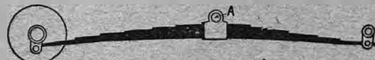
Fig. 16.—The Sheffield-Simplex rear spring, secured to the frame below a trunnion A.
