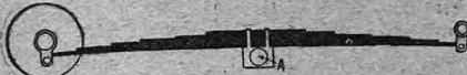
Fig. 15.—The Rolls-Royce rear spring. This is secured to the frame above a trunnion A.
