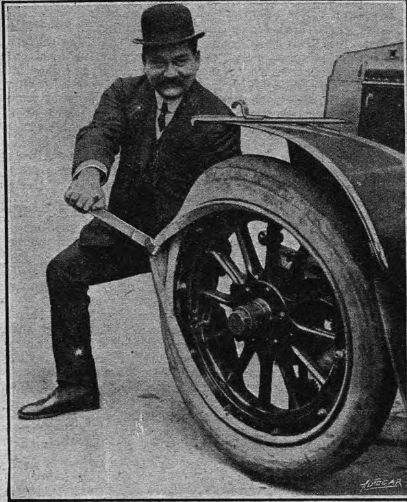
Fig. 1.—The Glentworth tyre lever in use. A second lever is shown on the wing of the car; it will be noticed that the lever extends beyond the hook for the tyre bead to enable it to reach the inner side of the rim which acts as a fulcrum.
