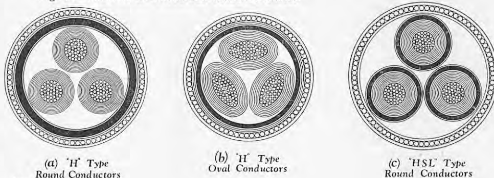
Fig. 1. SOLID PAPER-INSULATED SCREENED CABLES.
