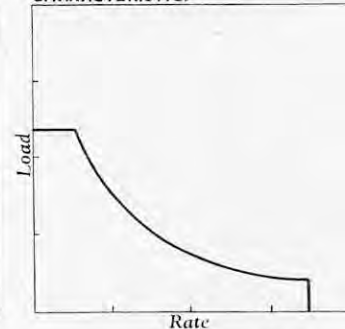
Fig. 6. CONSTANT-WORK PUMP CHARACTERISTIC.
