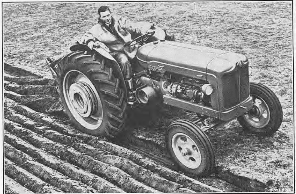
FIG. 1. TRACTOR FITTED WITH FORD-RANSOME MOUNTED PLOUGH.
