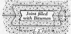
Fig. 7. PLAN OF SEAL IN VERTICAL JOINTS OF DOCKWALL.
